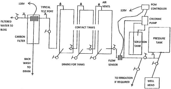
All sample taps (test ports) to be terminated with a smooth non threaded outlet.
