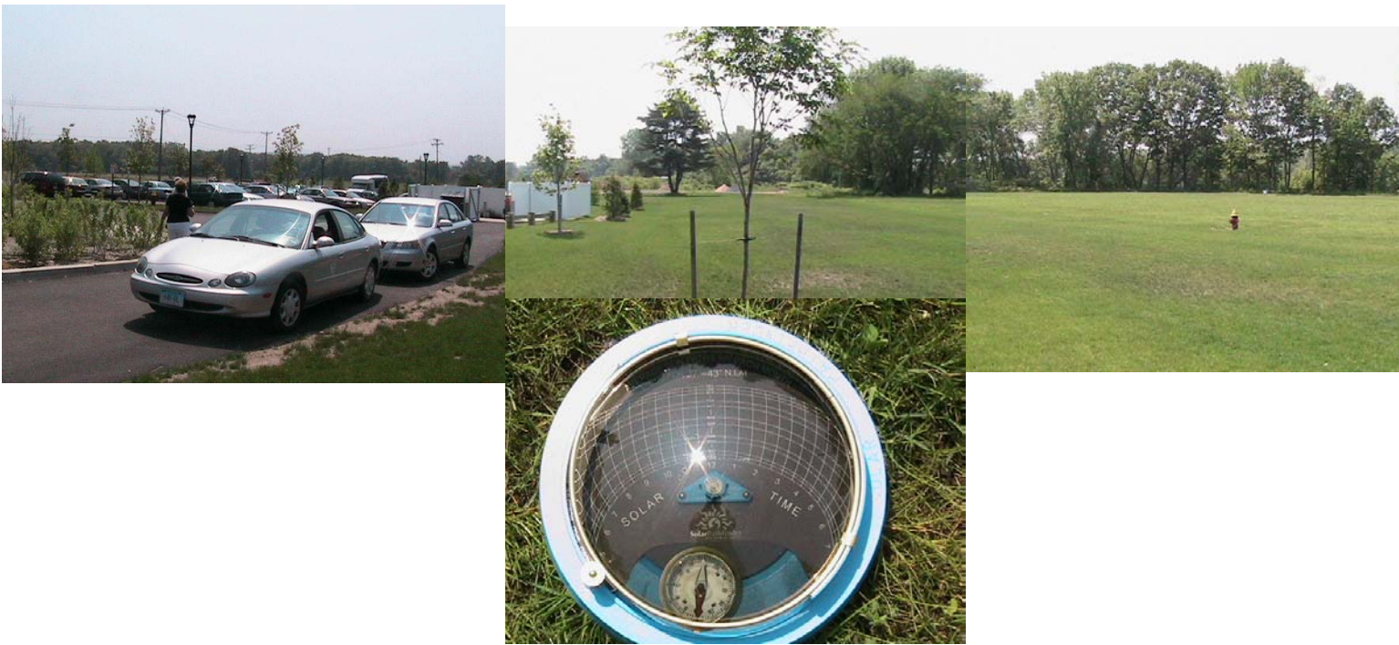
Fig 13: Southerly view from ground below optimal roof location and pathfinder image
