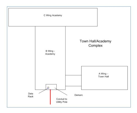
**Fiber Termination Location**: The cable will enter via underground conduit and terminate in a new rack mount enclosure in the Demarc Room. The other end routes all the way back to Glastonbury High School and routes into the Splice Cabinet. The conduit to the street is less than 200' and the demarc room is about 12'X18'.
