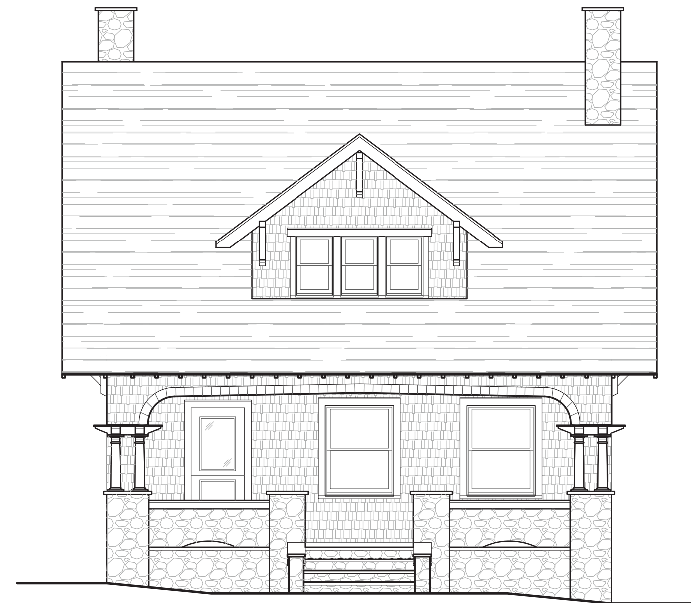
1.3 WEST EXTERIOR ELEVATION 1/4" = 1'-0"
