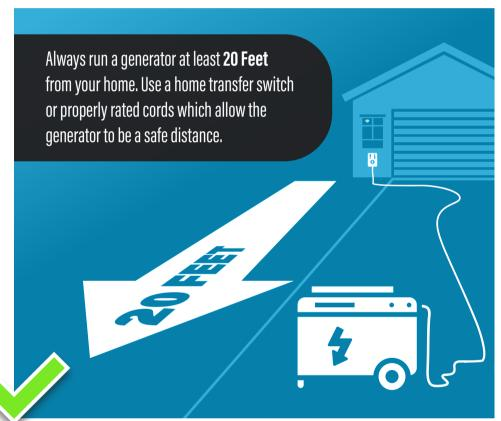
**DO NOT** wire a generator directly to home wiring or sockets. Bypass or improper wiring can cause damage or injury in the home or with power line technicians.
