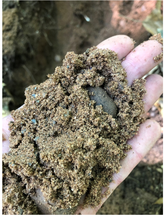
TP-2 Soils - red-brown medium to fine sand with little gravel and trace cobbles
