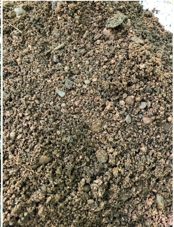
TP-3 Soils - red-brown fine to coarse sand with little gravel
