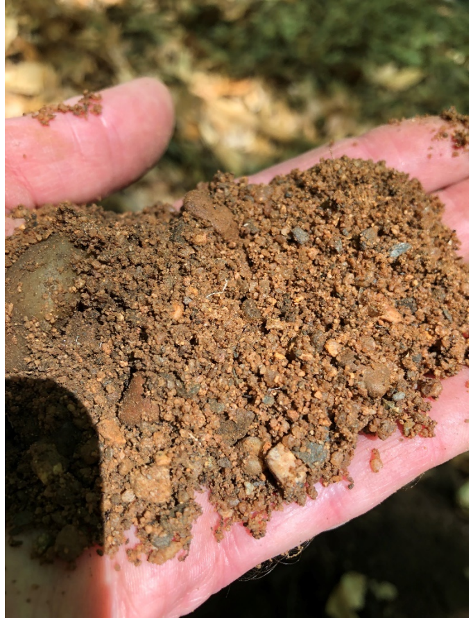
TP-1 Soils - dark red-brown coarse to very coarse sand with some gravel and few angular cobbles
