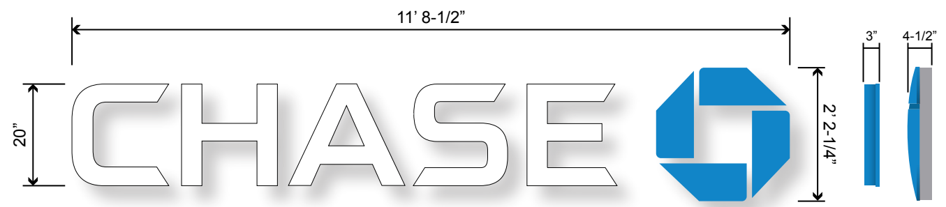
LIF-WBO-20-LED WHITE W/ BLUE OCTAGON ILLUM CHANNEL LETTERS - 25.6SF SCALE: NTS
