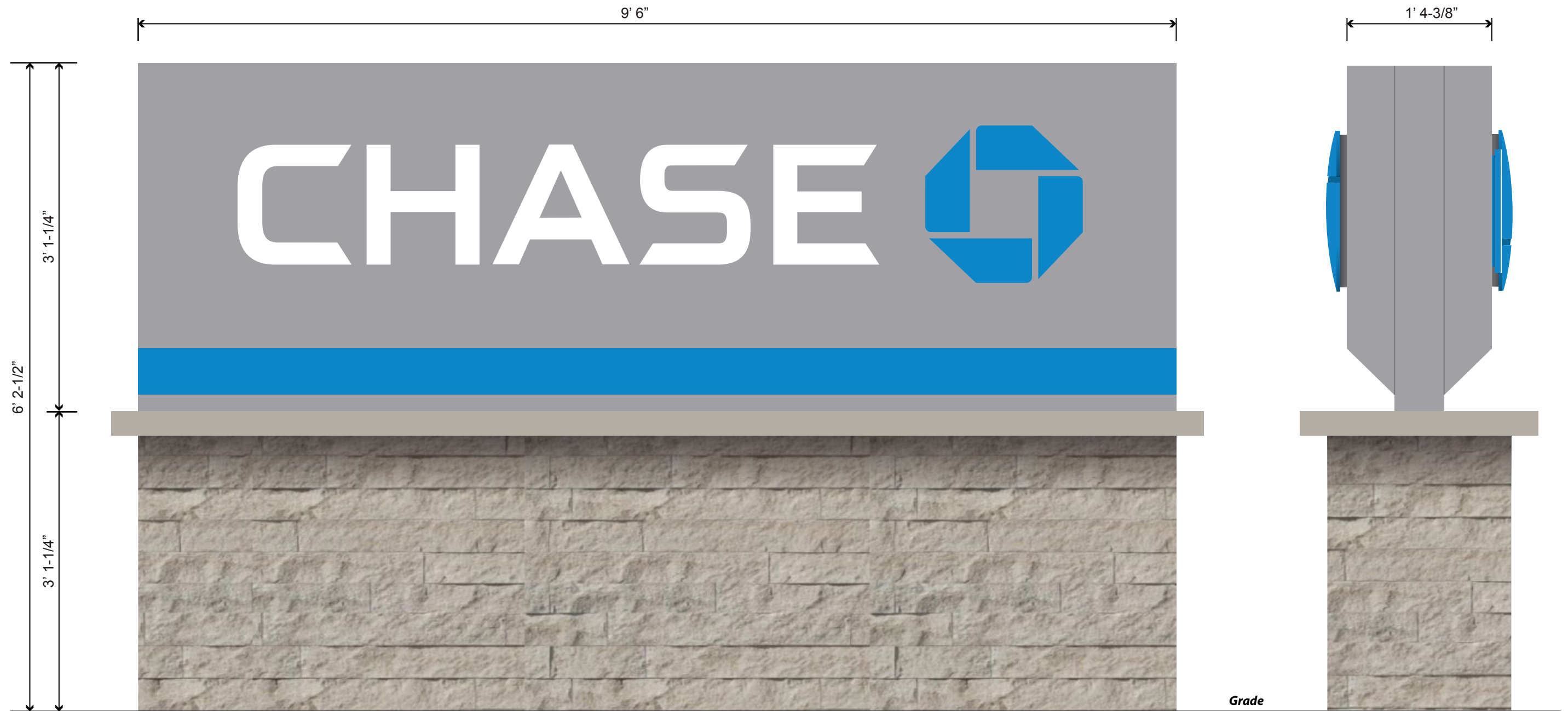
M-25-RE DOUBLE-FACED ILLUMINATED MONUMENT - 25SF SCALE: NTS
