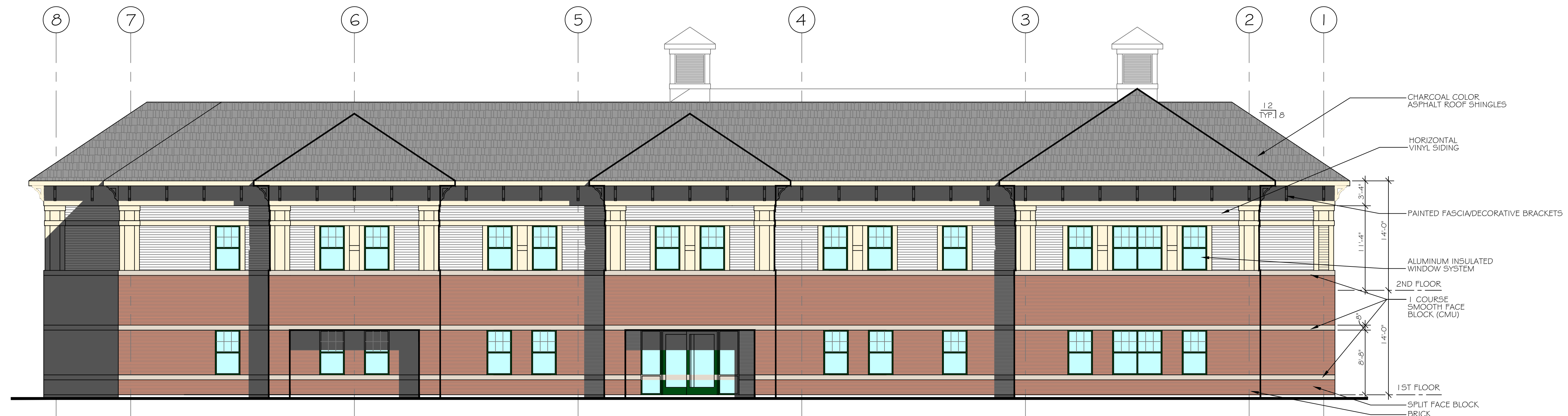
3 EAST ELEVATION (REAR) 1/8" = 1'-0"
