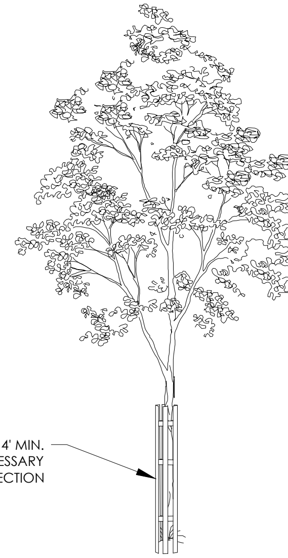
I TREE TRUNK PROTECTION DETAIL NOT TO SCALE
