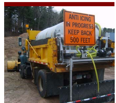
Brine equipment installed on plow truck
