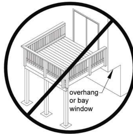
Figure 18. No Attachment to House Overhang with Ledger.
