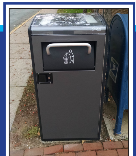
Refuse division installed a "Big Belly Compactor" outside of Town Hall's main entrance. This recycling solution uses solar energy to compact deposited waste and holds 5x the capacity of a standard garbage can.
